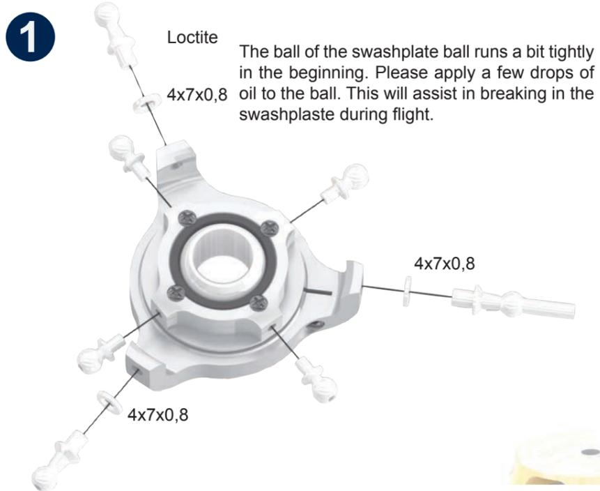
The ball of the swashplate ball runs a bit tightly in the beginning. Please apply a few drops of oil to the ball. This will assist in breaking in the swashplate during flight.
