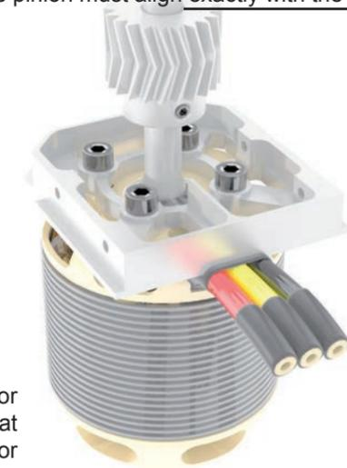
Please check that the end of the motor bolts do not go in too far. Ensure that there is a proper space between motor winding and cable.
