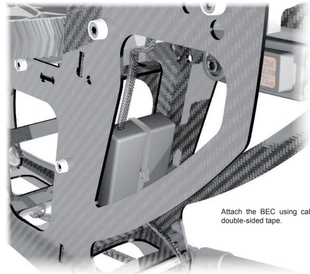
Attach the BEC using cable straps and double-sided tape.
