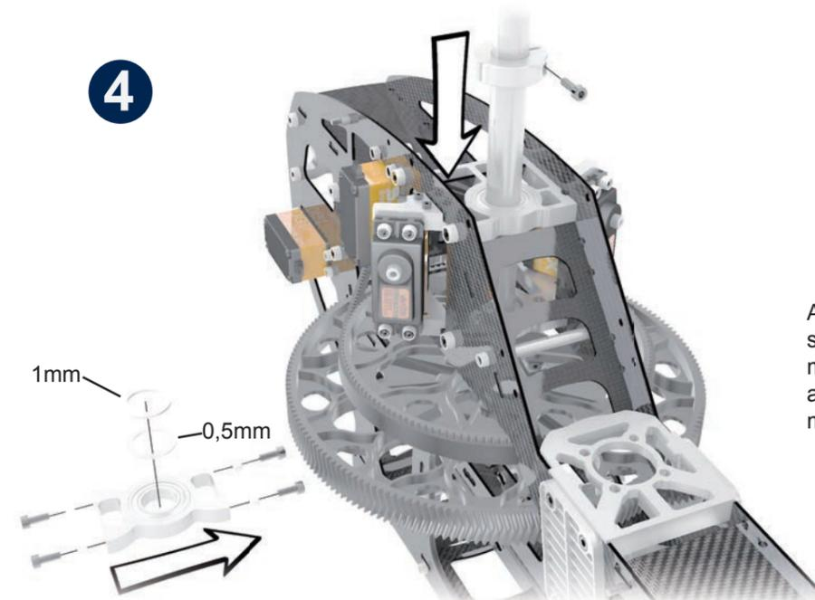
After mounting the main gear, it will show slight axial play. This is intended and will make installation of the pinion easier. It will also facilitate the correct setting of the gear mesh.
