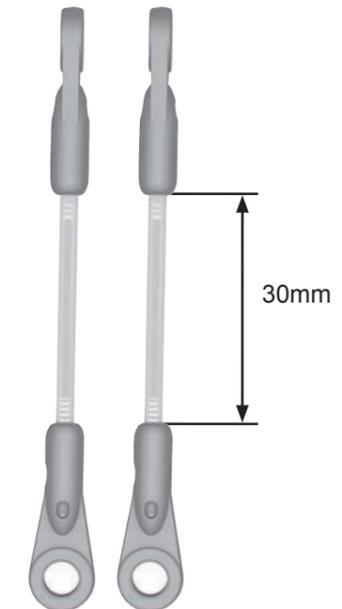
Note when mounting the ball links: If you find it hard to clip the ball link on, turn it 180°. One side of the ball link will clip on easily. The other one is too tight to clip on easily.
