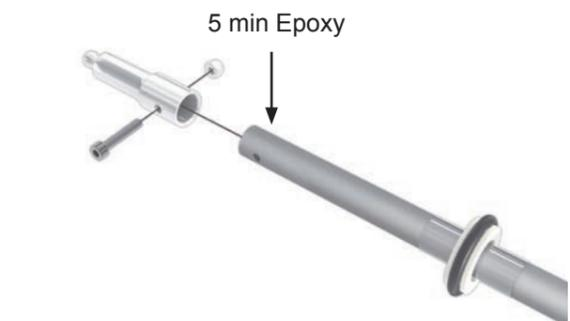
Before pushing in the torque tube, please ensure that the inside of the boom is clean. If necessary, clean it out with a piece of cloth.
