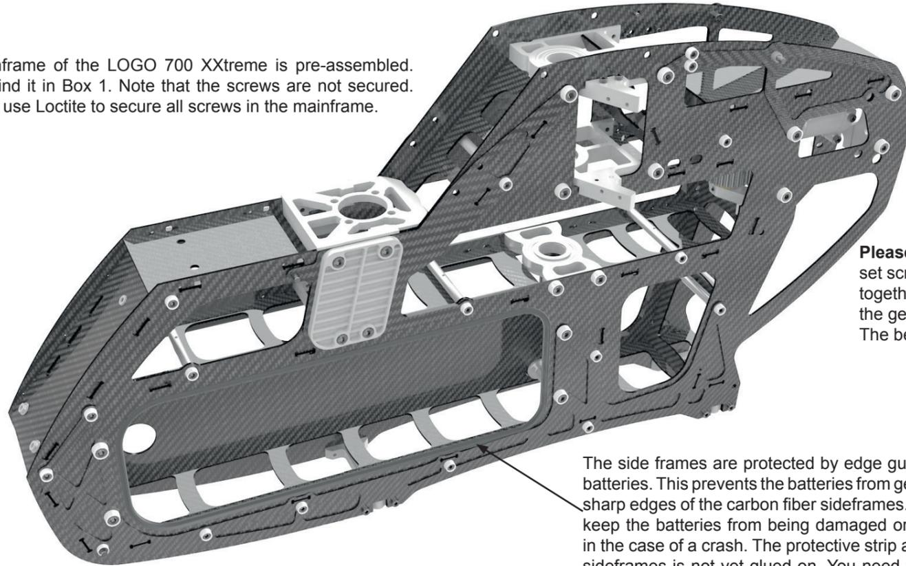
Please check if the RC-plate is fitted tightly between the frames, so that it cannot move. If the RC-plate is loose, please apply glue (CA glue or 5-min epoxy) to fix. A moving RC-plate can lead to vibrations and malfunction of the gyro sensor!
