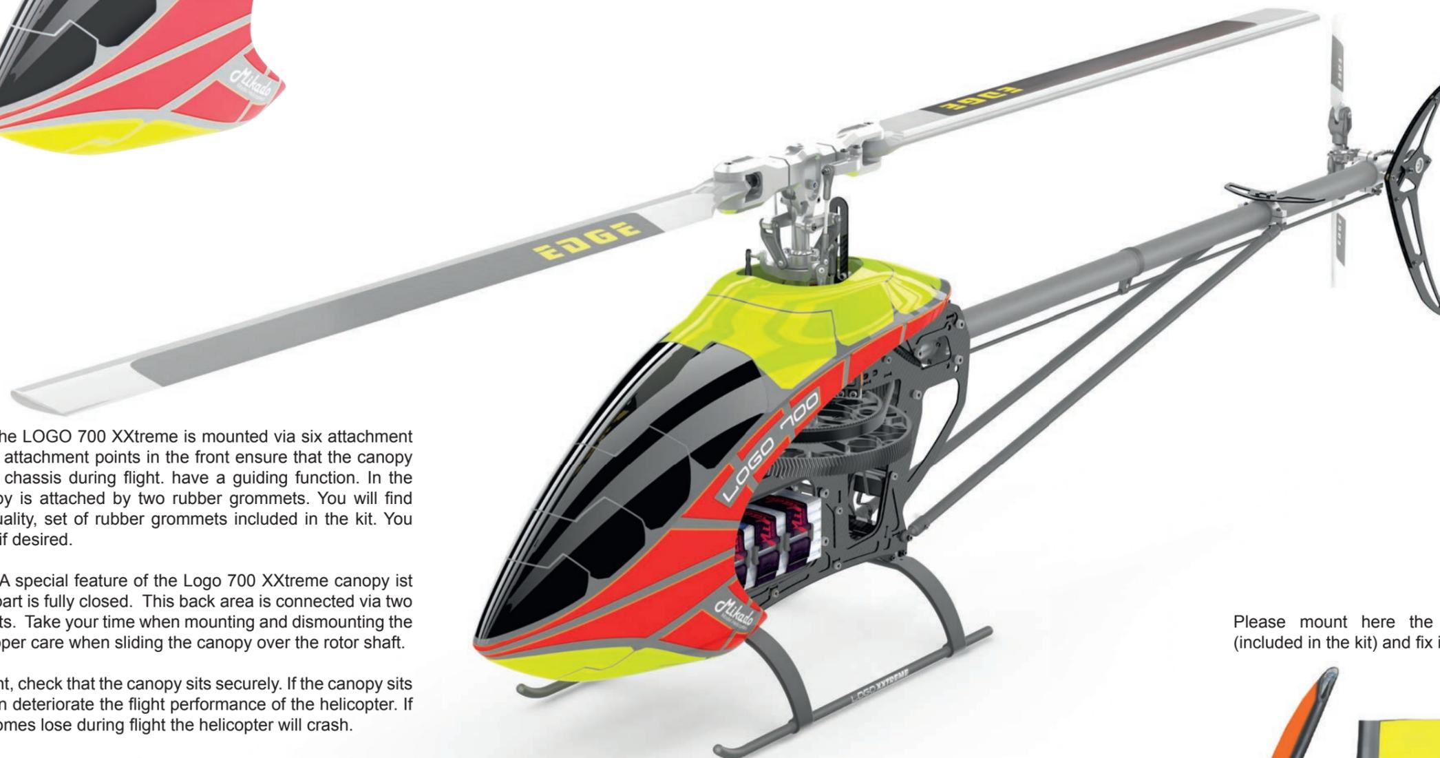
The canopy of the LOGO 700 XXtreme is mounted via six attachment points. The four attachment points in the front ensure that the canopy sits well on the chassis during flight. have a guiding function. In the back, the canopy is attached by two rubber grommets. You will find another, high-quality, set of rubber grommets included in the kit. You may use these, if desired.
