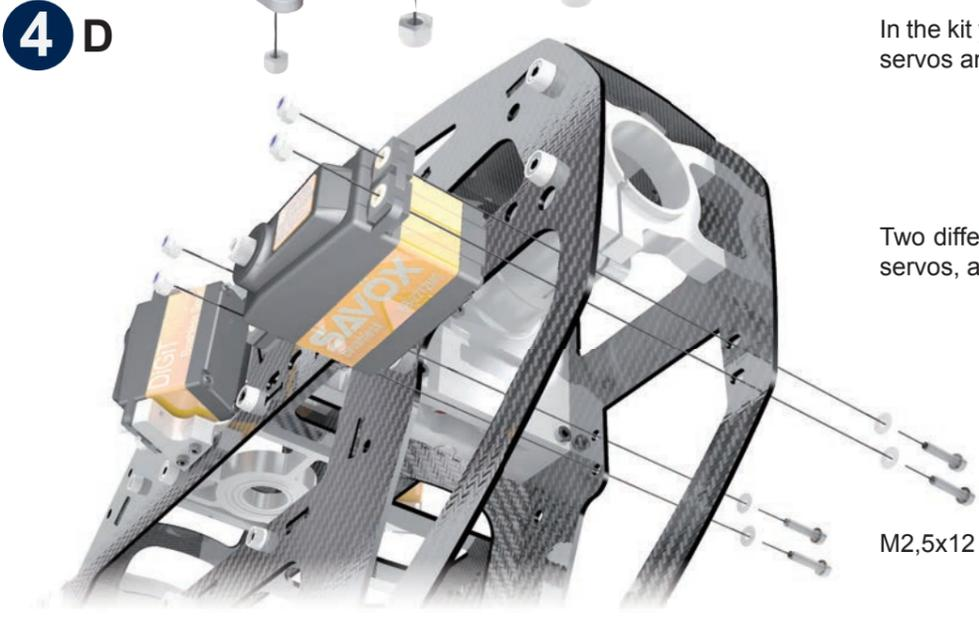
In the kit you will find servo mounting sets for Futaba/JR HV (11mm) servos and Savox HV (10mm) servos
